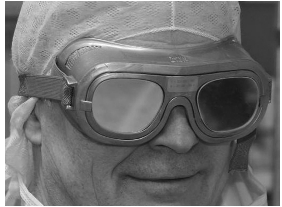
Figure 10.8 Safety goggles must either reflect or absorb the wavelength of the laser light in use.
